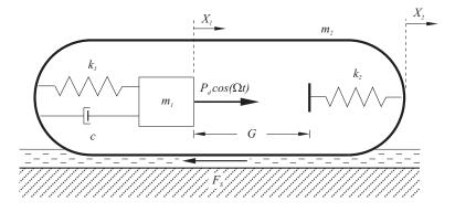
Figure 1: Physical model of the vibro-impact capsule system
