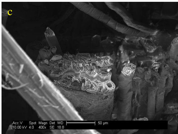
Figure 10: Overview of the fracture surfaces of flax/PLA tensile specimens
