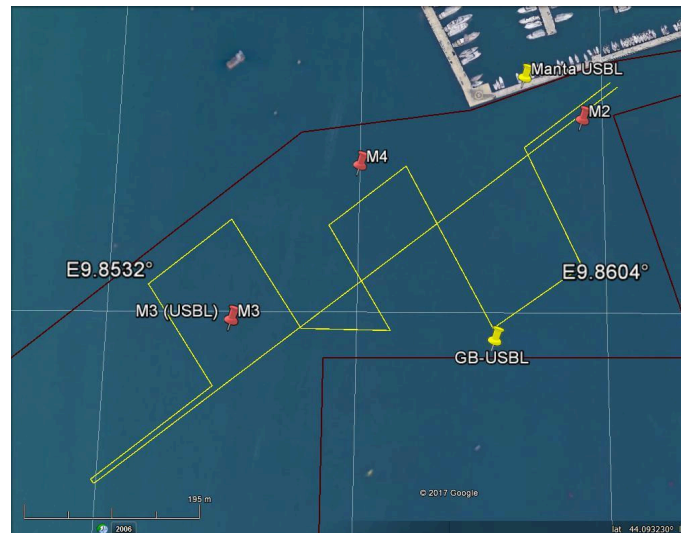
Fig. 4: Lawn mower and line trajectory. The mobile node starts the trajectory at the top right part of figure. It first follows the line trajectory and then returns following the lawn mower pattern.
