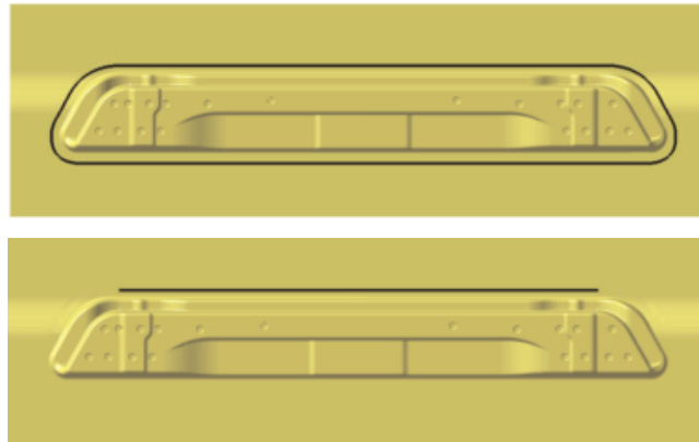
Figure 2.13 Beadless stamping proposal, original draw bead route (top) and modified draw bead (bottom). Image from Shim, (2013). Shim proposes replacing draw beads which surround the perimeter of a part, with an optimum blank shape which controls the material flow with less scrap, one draw bead is required to prevent oscillation in the part.
