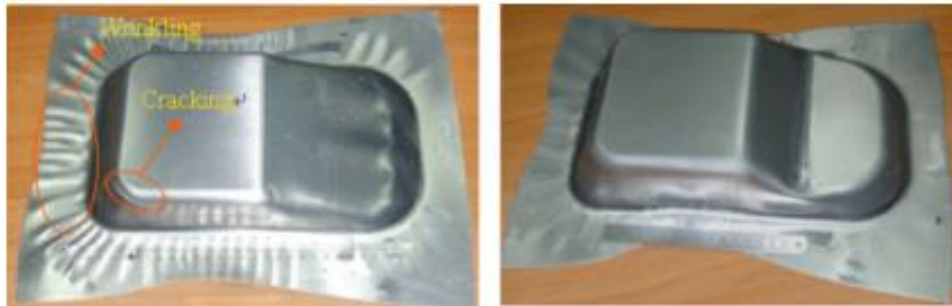
Figure 2.7 Improved forming results using control systems for time variable blank holder force Zhong-quin et al. (2007). This can be a successful method of forming, but it does not give understanding of how the blank and part geometry impacts the blank holder force.
