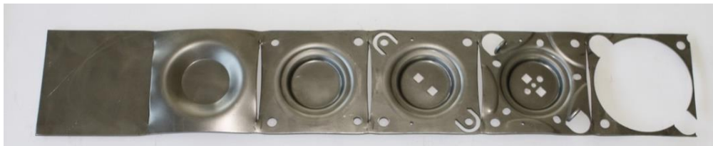
Figure 2.26 Use of slits to control material flow in progressive stamping. Image from Comec (2016).
