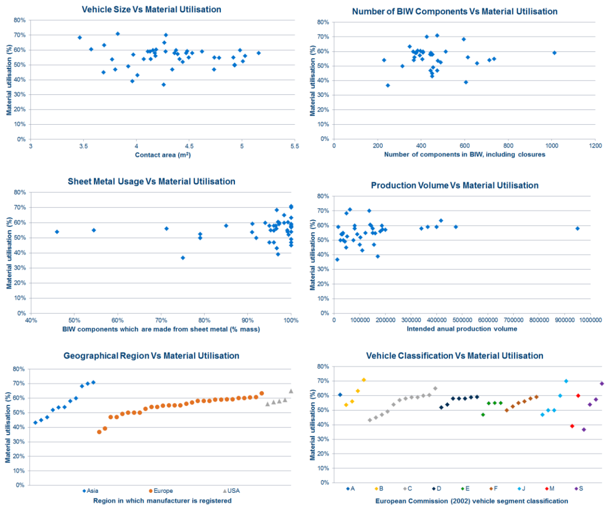
Figure 3.2 Plotting material utilisation values against vehicle attributes to identify trends.
