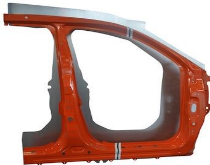
Figure 2.25 An automotive body side part and blank with a cut out. This part was developed for tailored welded blanks and has minimised material utilisation, image from European Aluminium Association (2013).
