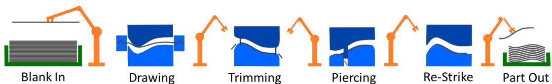
Figure 1.5 The stamping process. Scrap is generated to allow material to flow in the drawing process and is removed in subsequent trimming operations.
