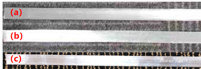
Fig. 4.6 Photo of the three types of superconducting coated conductors used in the experiment. (a) SSTC 23 g tape, (b) SSTC 28 g tape, (c) AMSC 23 g tape.
