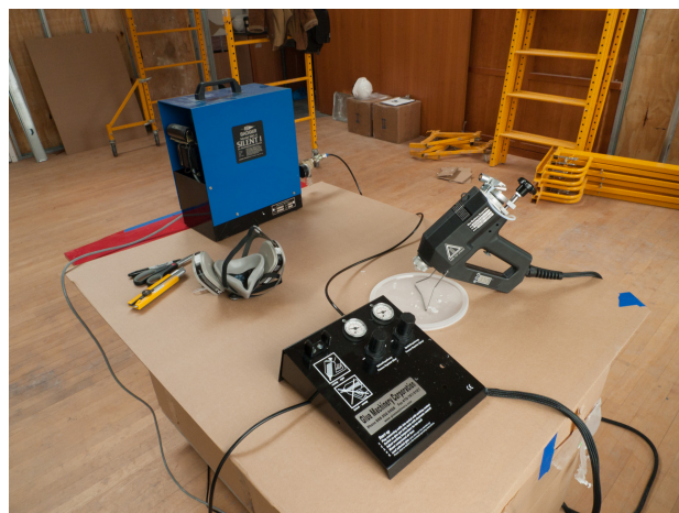
Figure 7 The Champ 10S LCD Hot Spray Gun, a device normally used to spray hot-melt adhesives. Photo: ©President and Fellows of Harvard College, photographed by the Straus Center for Conservation.
