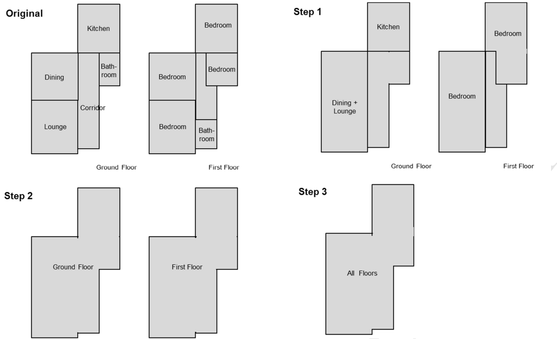
Figure 2 Incremental simplifications in thermal zoning
