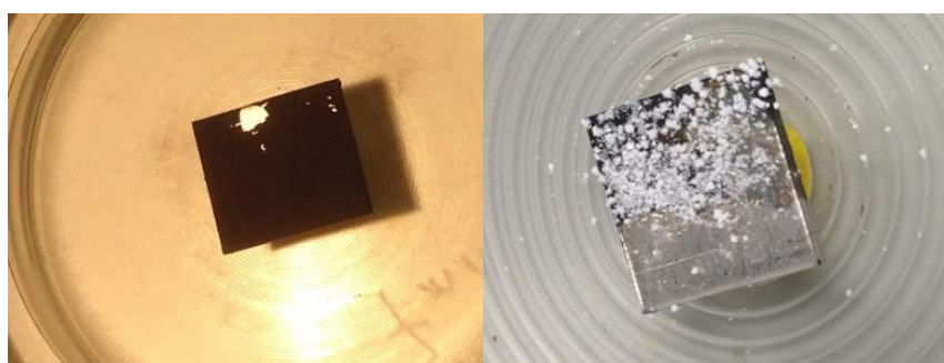
Figure 4.7 Optical images of PPy-coated steel substrate (left hand side) and MOF crystals on a semi-coated substrate (right hand side). MOF crystals were immobilised on the coated part whereas the majority of MOF crystals on the bare steel surface disappear during the transfer. The figure is reprinted under a Creative Commons Attribution 3.0 Unported Licence (CC BY 3.0) from ref. 114 (Copyright 2017 The Royal Society of Chemistry).
