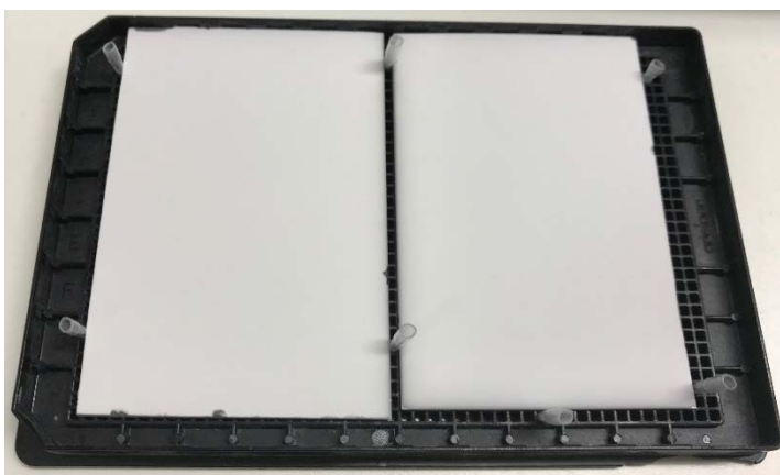
Figure 46: TLC-plates pegged onto 1536-well plate for HT-TLC assay.
