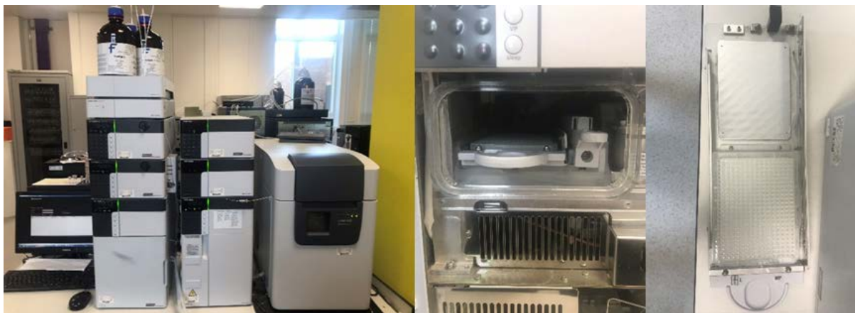
Figure 27: LCMS 2020 by Shimadzu in the Gaunt group. A) The overall setup of the LCMS; B) Autosampler with MTP-tray on left and controller rack on right; 3) MTP-tray with 384-well plate in position.
