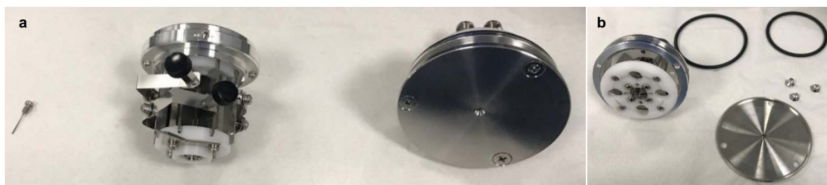
Figure 34: a) Corona Needle, Octopole, Skimmer and pre-quad assembly, b) disassembled pre-quad assembly.
