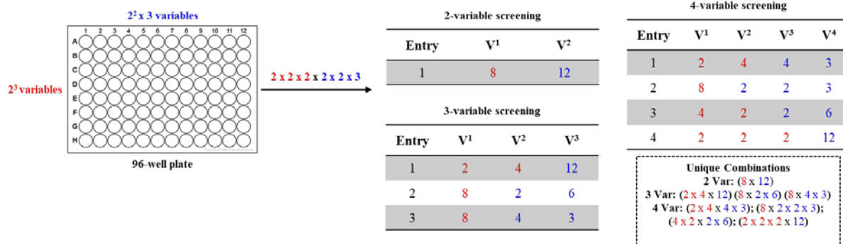
Figure 18: Example combinations for screening on a 96-well plate. Any permutation of these combinations can be used and are thus referred to as unique combinations.
