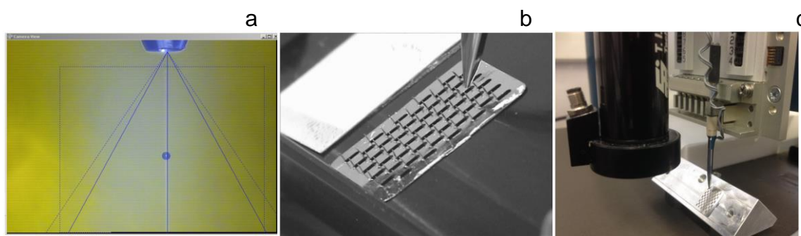
Figure 1.8. Inkjet coating of metallic microneedles array. (a) Drop diameter measured by a stroboscope. (b) MN positioned on a holder at an angle of 45°. (c) the overall image of the coating process (Modified from Uddin et al. 2015).
