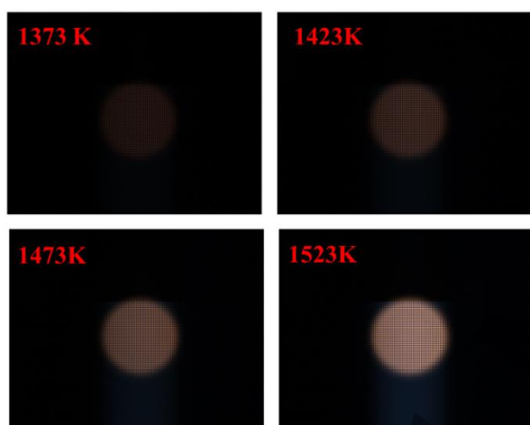
Figure 10. Example of the blackbody furnace images under different temperature settings
