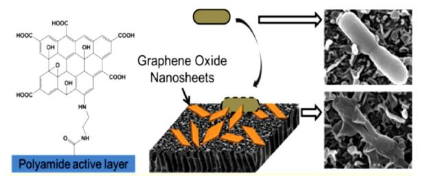
Figure 17: Functionalization of graphene oxide nanosheets onto the TFC membrane. The top SEM image shows normal E.coli cells on the membrane surface while the bottom SEM image shows compromised bacteria cells after membrane functionalization [280]
