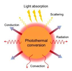
Figure 2: Schematic of photothermal conversion. Reproduced from [52] with permission from The Royal Society of Chemistry
