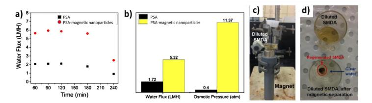
Figure 11: (a) Graph of FO water flux v/s time, (b) comparison of average water flux and osmotic pressures generated by of PSA and PSA coated magnetic nanoparticles (c-d) Magnetic separation of SMDA.
