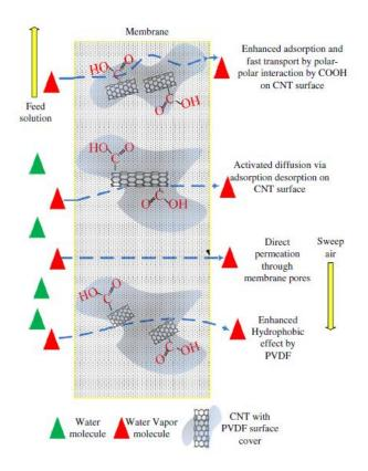
Figure 20: Mechanism action of c-CNTs in MD [372]
