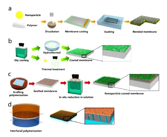
Figure 14: Antibacterial membrane preparation process: (a) Blending (b) surface coating (c) surface grafting d) interfacial polymerization [239].
