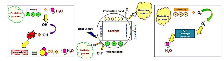
Figure 1: Schematic representation of a photocatalytic mechanism utilizing semiconductor photocatalysts [42]
