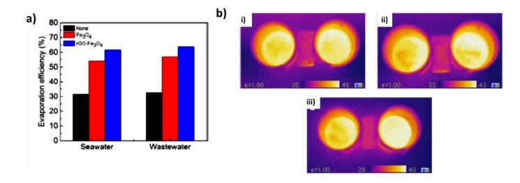
Figure 12: a) Evaporation efficiency of seawater and wastewater with dispersed Fe<sub>3</sub>O<sub>4</sub> and rGO-Fe<sub>3</sub>O<sub>4</sub> magnetic nanoparticles (b) IR images of the separation process [221].
