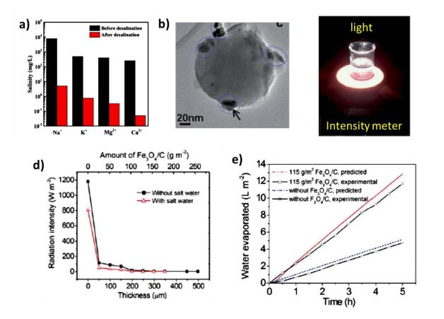
Figure 8: (a) Measured salinity of four primary ions before and after solar desalination, reproduced from [169] with permission from The Royal Society of Chemistry, (b) TEM image of a  $Fe_3O_4/C$  particle with the  $Fe_3O_4$  nanoparticles circled in blue, (c) Testing setup, (d) The radiation intensity measured underneath the
