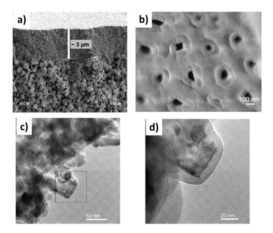
Figure 4: (a) SEM cross-section of a  $3\mu$ m TiO<sub>2</sub> layer deposited on an alumina support [98] (b) SEM image of the TiO<sub>2</sub> nanotube membrane after 2 h of grafting [99], (c) TEM and (d) HRTEM images of HAP-supported Ag–TiO<sub>2</sub> composite [100].
