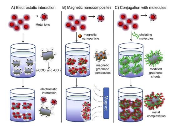
Figure 22: Main strategies to apply graphene-based materials as adsorbents for metal ion removal (A) electrostatic interaction; using non-modified graphene, GO or rGO, (B) magnetic attraction; Graphene sheets can be functionalized with magnetic nanoparticles to improve adsorption capacity and (C) synergetic effect between the chelating properties of the organic molecules and adsorption capacity of the graphene sheets. Reproduced from [365] with permission from The Royal Society of Chemistry.
