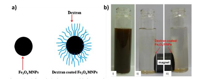
Figure 10: (a) Schematic showing dextran coated  $Fe_3O_4$  magnetic nanoparticles (b) Demonstration of separation of these nanoparticles when (i) the particles are well dispersed in the solution, (ii) the separation situation of these nanoparticles MNPs containing with 64.44 wt.% dextran after 10 min and (c) 78.03 wt.% dextran after 15 min. [197]
