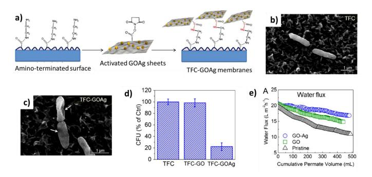
Figure 19: (a) Schematic illustrating the formation of GO/Ag-TFC membrane, (b) SEM image of bacteria cells attached to the TFC-GO membrane (c) SEM image of bacteria cells attached to the GO/Ag-TFC membranes, (d) Viable cells of P. aeruginosa after three-hour contact with the surface of pristine and graphene modified membranes and (e) Water flux decline for TFC, GO-TFC and GO/Ag-TFC membranes [348].
