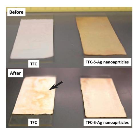
Figure 15: Difference in E. coli biofilm growth on TFC and Ag grafted TFC (TFC-S–Ag nanoparticle) membranes after 7 days [253]
