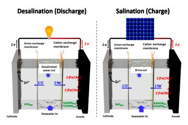
Figure 7: Schematic of the desalination battery operation during desalination (discharge) and salination (charging) [149].
