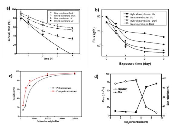
Figure 3: (a) Photocatalytic bactericidal effects of the TiO2 hybrid and neat aromatic polyamide membranes in the dark and with UV illumination [85]. (b) Water flux of the hybrid and the neat LP membranes with and without UV light after exposure to microbial cells [86]. (c) Rejection profiles of PES and nanocomposite membranes [84] and (d) Effect of TiO2 concentration on the membrane performance of water flux and MgSO<sub>4</sub> rejection (MgSO<sub>4</sub> concentration was 2000 ppm).
