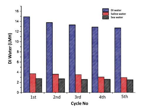
Figure 23: Water fluxes for the various feed solutions after each cycle after regeneration using Fe<sub>3</sub>O<sub>4</sub> magnetic nanoparticles grafted with PSSS-PNIPAM draw solute. Reprinted with permission from Zhao et al. [200], Thermoresponsive magnetic nanoparticles for seawater desalination, ACS Applied Materials and Interfaces, Copyright (2013) American Chemical Society.
