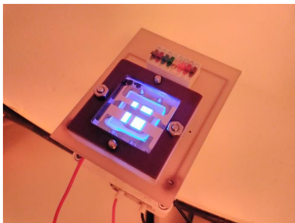
Figure 3.8. Blue OLED device at work.
