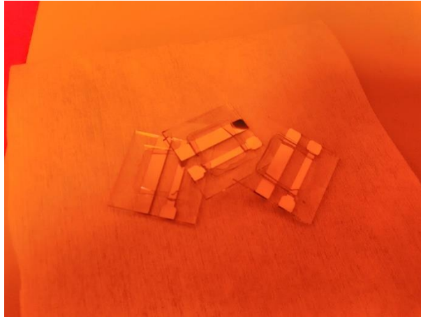
Figure 3.7. Encapsulated OLED devices.
