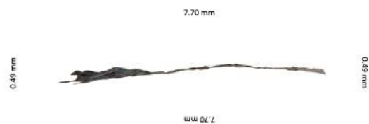
Figure 3.11: A2 (1/100 scale) seen from the vertical position. As the whole image forms a bowl-like concave shape, the elevation is highest at both ends, while the lowest surface is found in the middle part.
