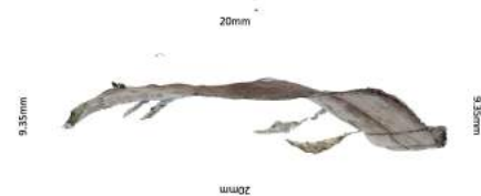
Figure 5.27: PB4 (1/30 scale) seen from the vertical position. The highest elevation is found on the hind limbs, while the lowest is on the central mid-torso.
