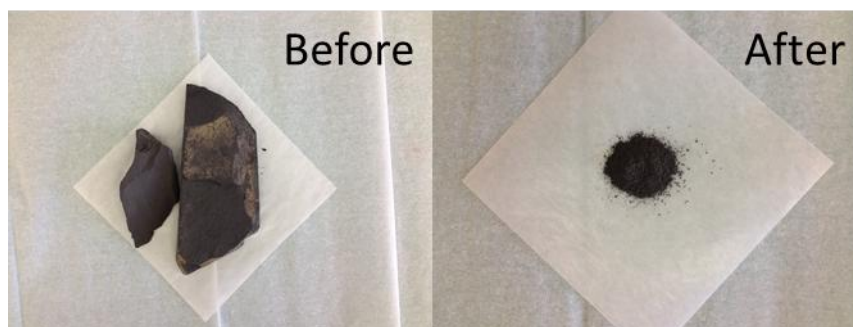
Figure 3.14 Photos of the gas shale sample before and after grinding.
