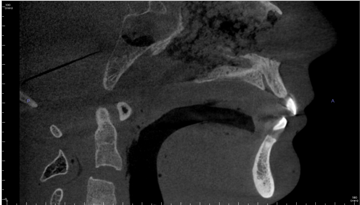
Figure 26: Hard palate in the sagittal view simulating the test tool location and orientation of the Mod1 Quart phantom at the 17x11 cm FOV, SDSR.
