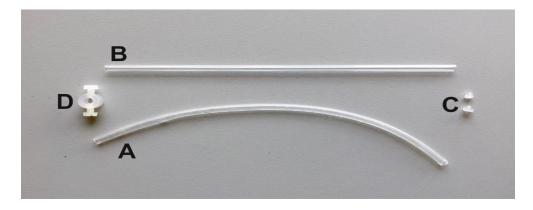
**Figure 13**: 5 mm stretching device designed by Kummerlöwe for all commonly used solvents. The device is composed of a Kalrez tube (A), an open cut 5 mm NMR tube (B), a specially designed Polychlorotetrafluor ethylene (PCTFE) screw (C) and a Kel-F/PCTFE cap with 2 screws (D).
