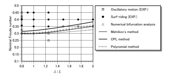
Figure 10 Comparison of the predicted surf-riding threshold for the three methods with the experimental results as functions of wavelength to ship length ratio for a wave-steepness of 0.05.
