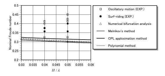
Figure 11 Comparison of the surf-riding threshold between experimental results and several methods as functions of wave-steepnessfor a wavelength to ship length ratio of 0.8.
