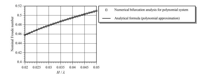
Figure 6 Comparison of the surf-riding threshold predicted using the Numerical Solution, and that predicted using the Analytical Solution with the polynomial approximation, for  $\lambda/L = 1.0$ .
