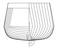
Fig.2 Body plan of the ONR tumblehome vessel.
