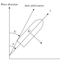
Figure 7 Definition of the heading angle and the autopilot course with respect to the wave direction.
