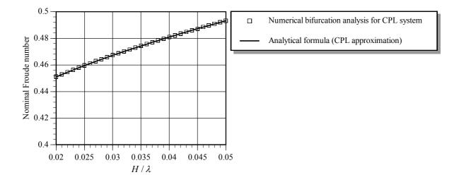
Figure 3 Comparison of the wave blocking threshold predicted using the Numerical Solution, and that predicted using the Analytical Solution with Piecewise Linear approximation, for  $\lambda/L = 1.0$ .
