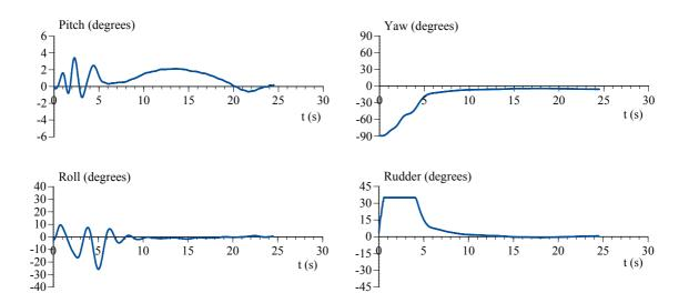
Figure 8 Time series of the oscillatory motion with Fn = 0.45 and  $\chi_c = -5.0$  (deg.) for  $\lambda/L = 0.8$ ,  $H/\lambda = 0.05$ .
