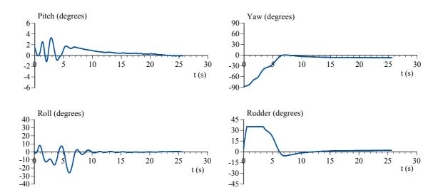
Figure 9 Time series of surf-riding with Fn = 0.4 and  $\chi_C = -5.0$  (deg.) for  $\lambda/L = 0.8$ ,  $H/\lambda = 0.05$ .
