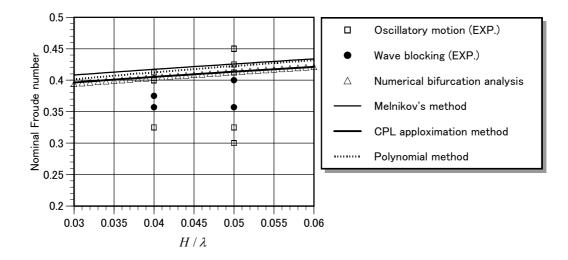
Figure 13 Comparison of the wave blocking threshold between experimental results and several methods as functions of wave-steepness, for a wavelength to ship length ratio of 0.8.
