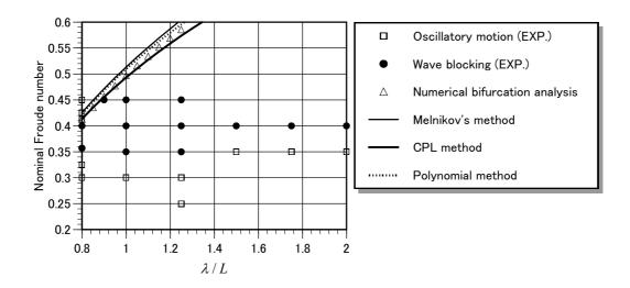
Figure 12 Comparison of the wave blocking threshold for the three methods as functions of wavelength and ship length ratio with the experimental results for a wave-steepness of 0.05.
