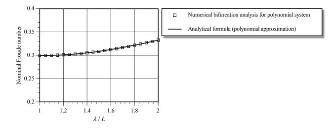
Figure 5 Comparison of the surf-riding threshold predicted using the Numerical Solution, and that predicted using the Analytical Solution with the polynomial approximation, for  $H/\lambda = 0.05$ .
