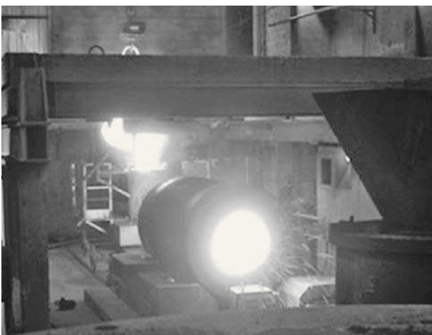
Figure 2 Centrifugal casting of the working shell
