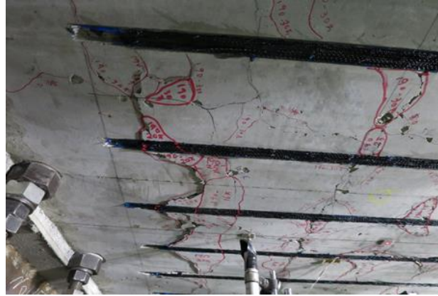
Figure 5.7 The fixing end of carbon fiber after experiment
