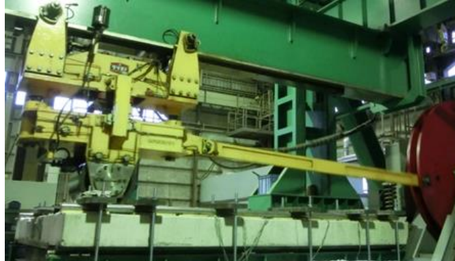
Figure 5.4 Crank type running test machine
