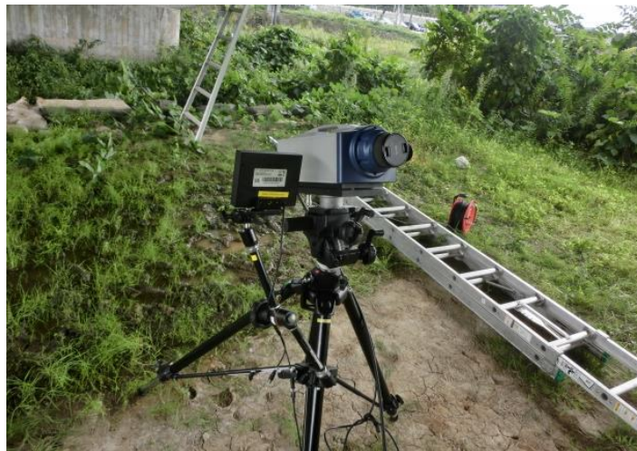
(a) Laser displacement meter under the bridge
