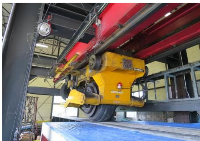
Figure 5.3 Wheel load running test machine
