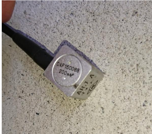
Figure 2.5: Acceleration meter (Tokyo Instrument ARJ-200A)
