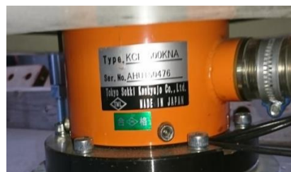
Figure 2.4: Load cell (Tokyo Instrument KCE-500kNA)
