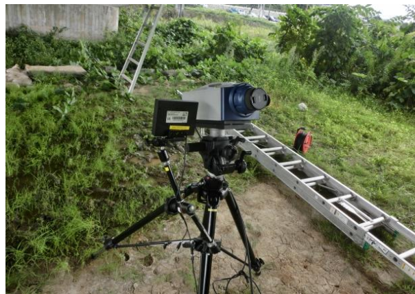
Figure 2.9: Laser displacement meter installation
