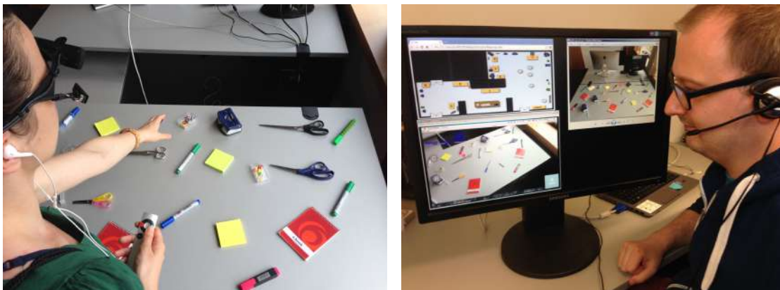
FIGURE 4.1: The experimental setup: the walker wearing a head-mounted eye tracker, following instructions and selecting objects (left picture) and the remote instructor giving directions, describing the next target and monitoring the walker's behavior (right picture)
