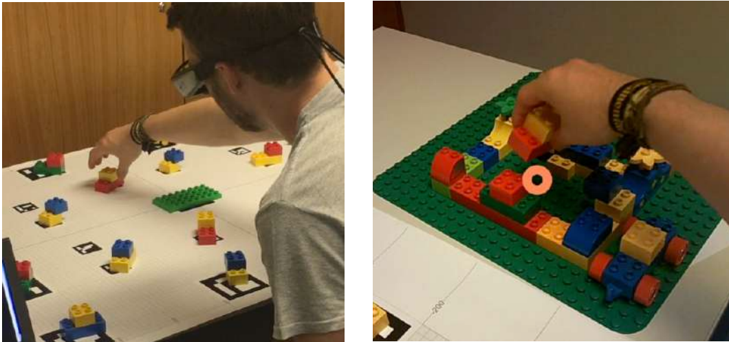
FIGURE 6.3: An example trial: System instructs the user by saying “Pick the big red building block.” The listener identifies and grasps it. After that it is assembled to the other LEGO blocks (right picture). The circle represents the gaze cursor.
