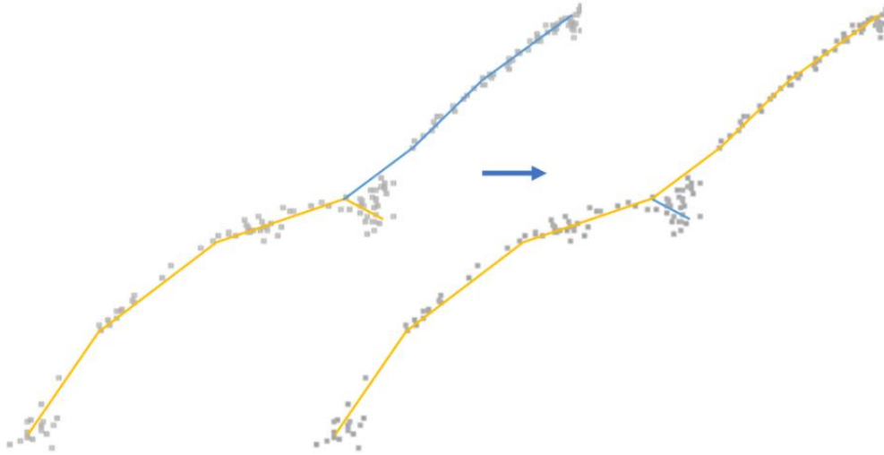
Figure 3.5 Example of branch connection refinement. Gray dots are scanned branch points, yellow and blue lines are connection lines. The right panel shows a more natural way of connection than the left.
