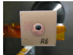
(a) Normal patch antenna (FR4 as dielectric)
