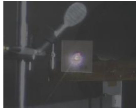
Fig. 10. Discharge emitting light on the surface of the patch antenna.
