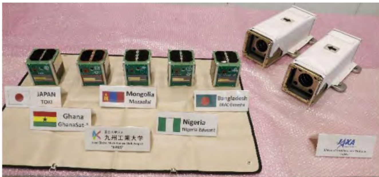
FIGURE 10. Five BIRDS-1 satellite with two J-SSOD.
