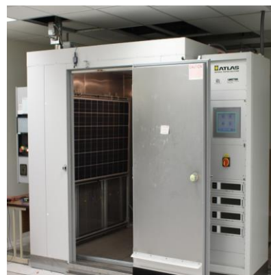
Fig. 1. Large-scale PV module environmental test chamber at UA.
