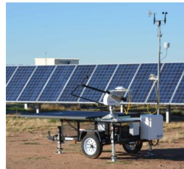
Fig. 5. SOFIE autonomous irradiance and weather measurement station.
