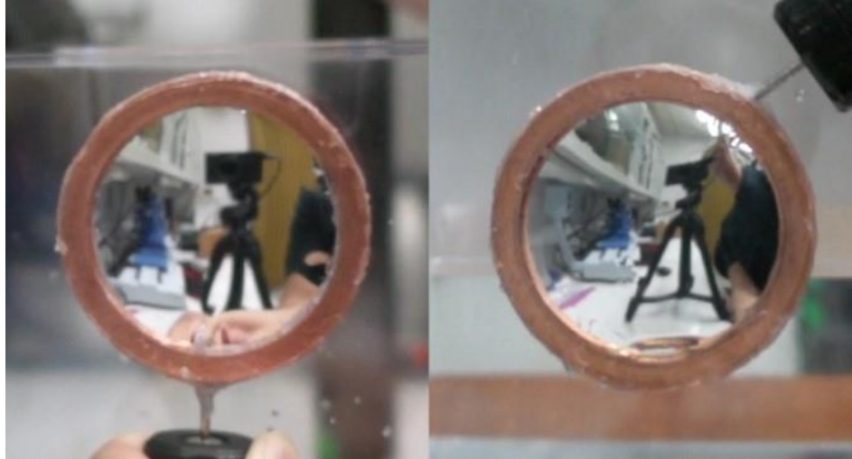
Figure 31. Left: Mylar Pre-Heat Treatment. Right: Mylar Post-Heat Treatment. Both images are taken of Mylar in air. A magnification change is noticed after Mylar had been subjected to heated water.
