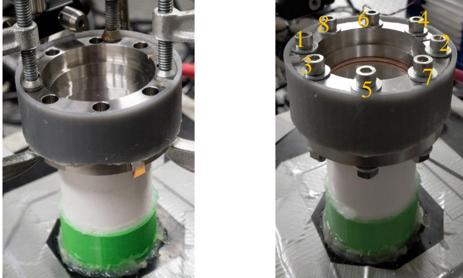
Figure 8. Mirror set up with three clamps holding flanges (left). Mirror set up with eight screws holding flanges (right). Numbers displaying order of tightening screws.
