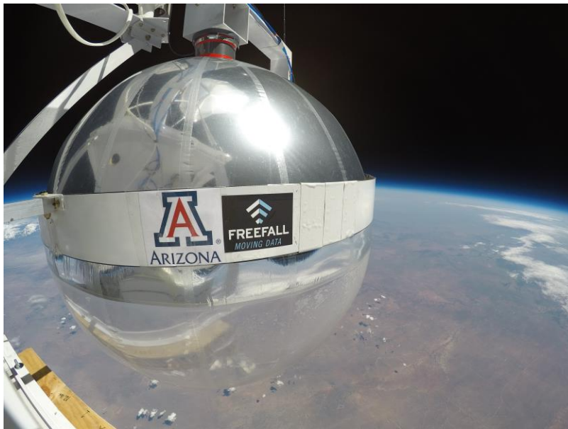
Figure 1. Image of stratosphere test flight with a 1-meter sphere for telecom. Image courtesy of C. Walker; funded by the Office of Naval Research and Free Fall Aerospace.
