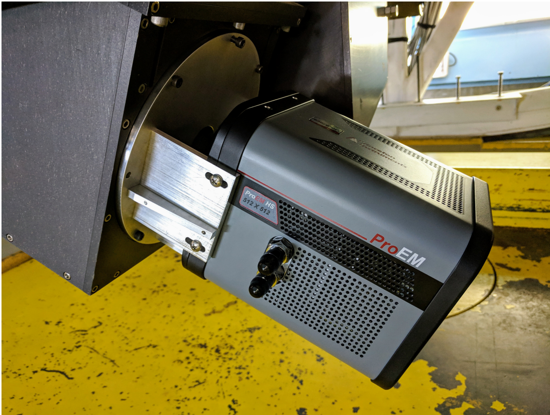
Fig. 3.1 — The EMCCD mounted to the Red Channel.
