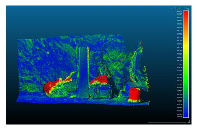
Figure 27 The result after performing change detection between test flight 11 and LIDAR scan 1
