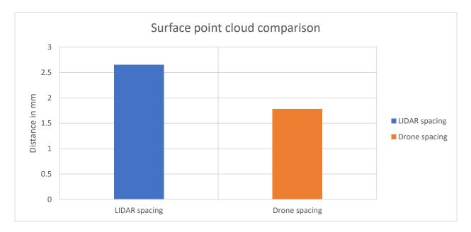
Graph 5: Comparison of point spacing between point cloud from LIDAR scan 2 and test flight 17
