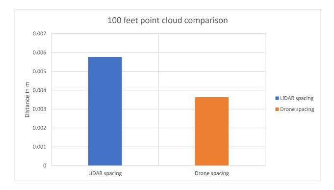
Graph 4: Comparison of point spacing between point cloud from LIDAR scan 1 and test flight
