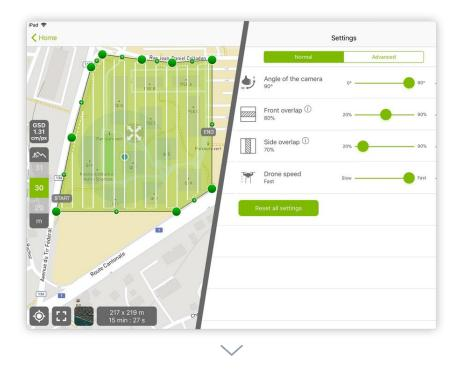
Figure 4 The first step of capturing image by using a drone for photogrammetry is setting up the path for the image capture. (Source: PIX4D support)
