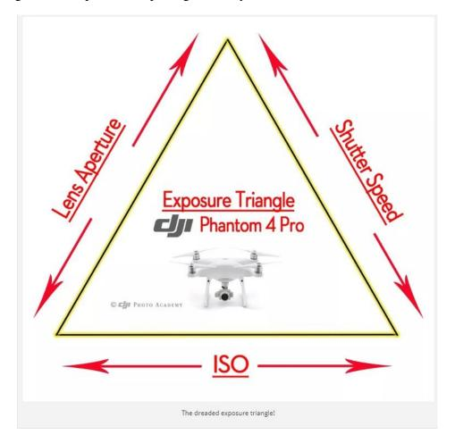
Figure 14 The Dreaded Exposure triangle shows the relation between lens aperture, shutter speed and ISO
