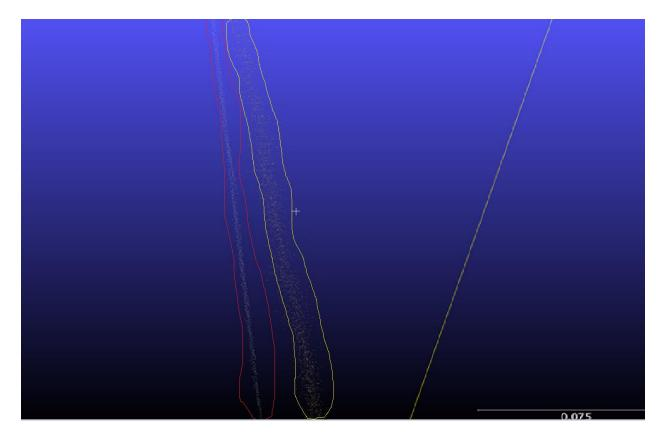
Figure 24 A comparison of the point cloud data of a flat surface for thickness. The red area is a point cloud from LIDAR and yellow is point cloud from the drone
