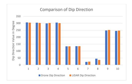
Graph 8: Comparison of Dip Direction value for plane generated in Drone and LIDAR point cloud
