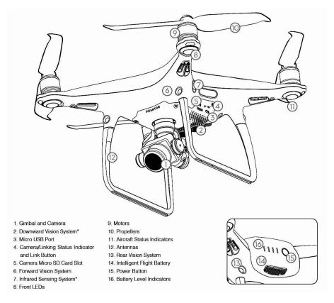
Figure 12 Different parts of the drone showing battery and camera gimbal
