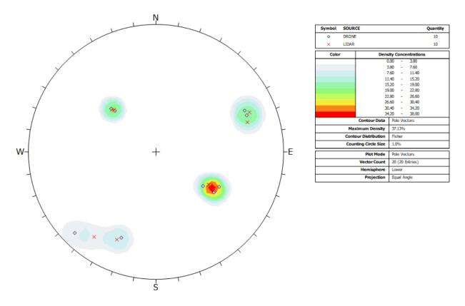
Figure 29 Stereonet projection of 20 different planes generated by Drone and LIDAR point cloud
