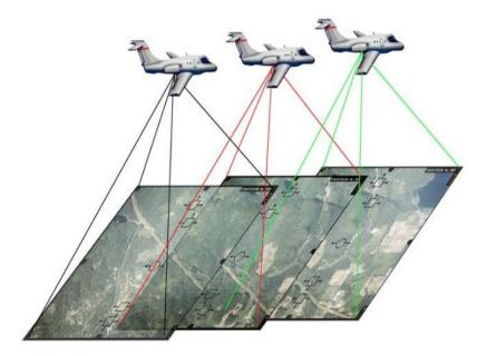
Figure 3 The above image demonstrates the basic principle of photogrammetry by mounting a camera on an airplane point towards ground. A series of overlapped images taken by camera is used to generate point cloud by using Structure from Motion (Sfm) method (Source: GIS Resources)
