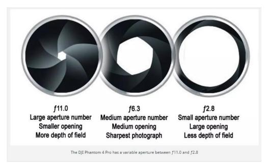
Figure 15 The value of the different aperture and the opening of lens at those aperture value
