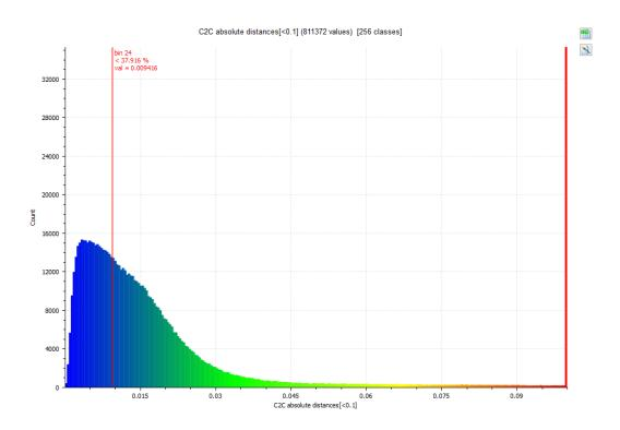
Figure 28 Histogram showing the distribution of point cloud scalar color after performing change detection.
