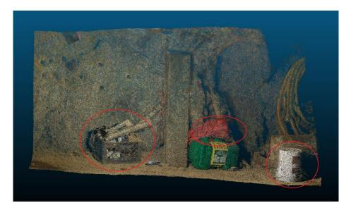
Figure 26 Drone point cloud from test flight 11 at 100 feet level at the SX Mine. The red circle shows the object that is not present in the LIDAR point cloud
