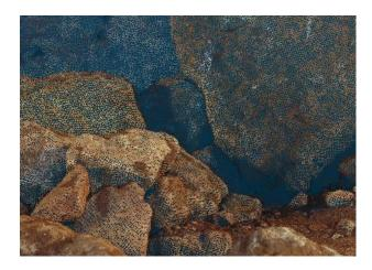
Figure 21 Voids in the point cloud after test flight 6
