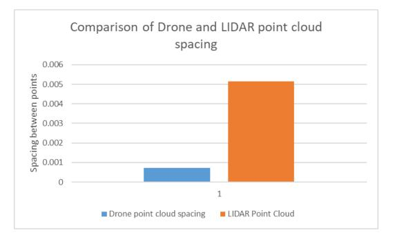
Graph 2: The graph shows the distance between point cloud generated by the drone during flight 11 and LIDAR point cloud (The value on Y-axis is normalized value and not in feet or centimeter)
