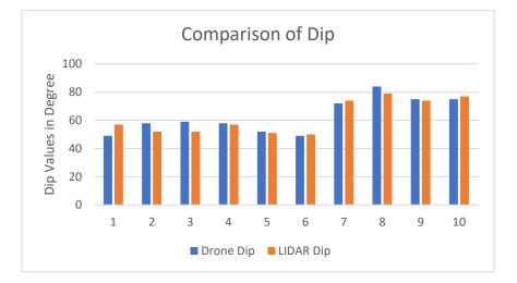
Graph 7: Comparison of Dip value for plane generated in Drone and LIDAR point cloud
