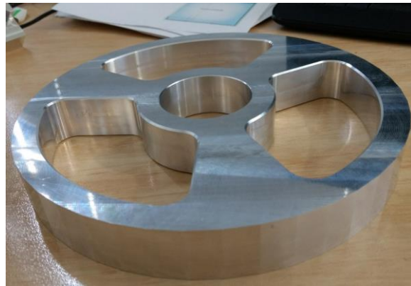
Fig. 43. Faceted polygon milled from aluminium, 200 x 28mm.
