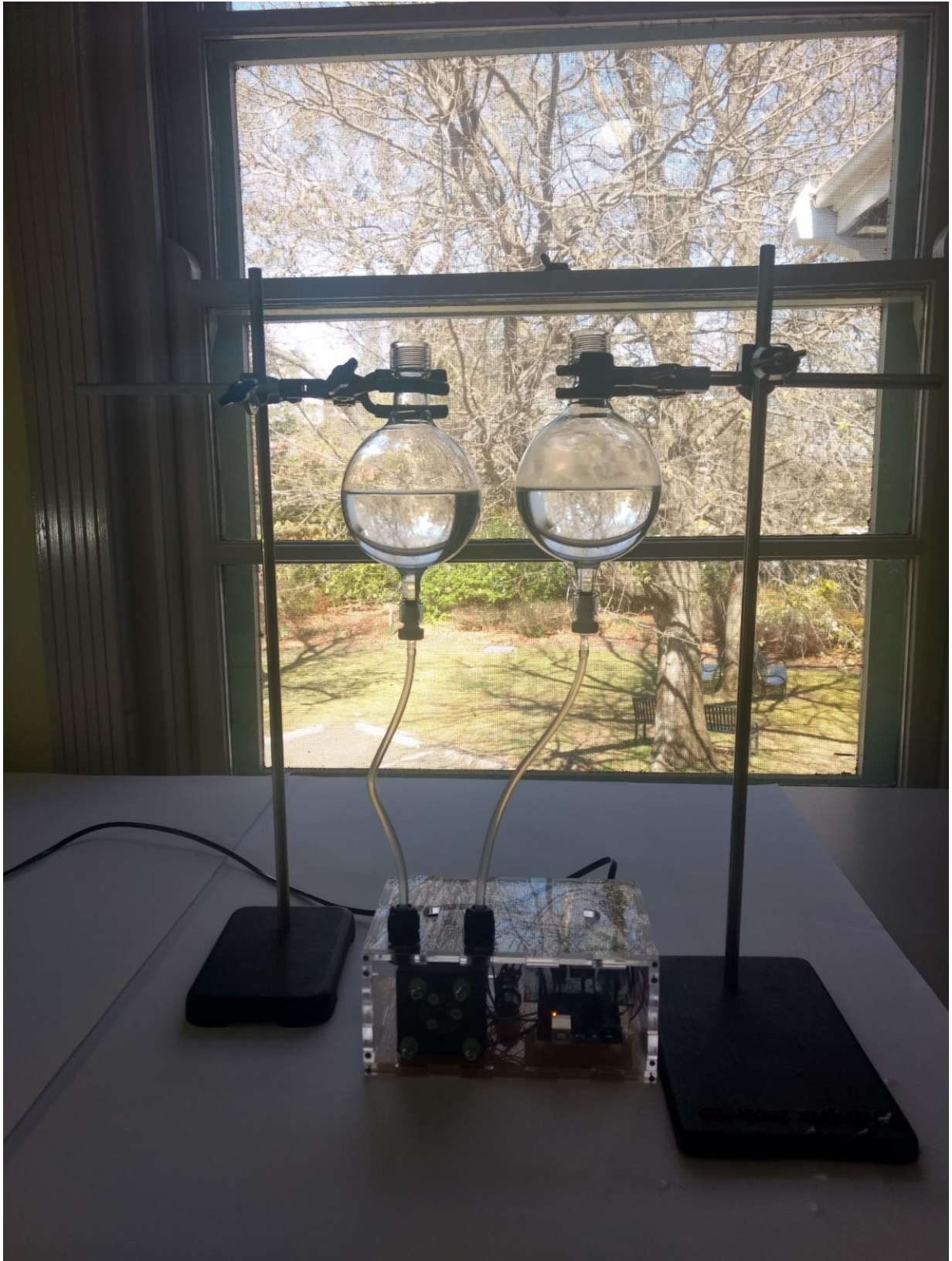
Fig. 19. Hollow lenses with exposed pump mechanism.
