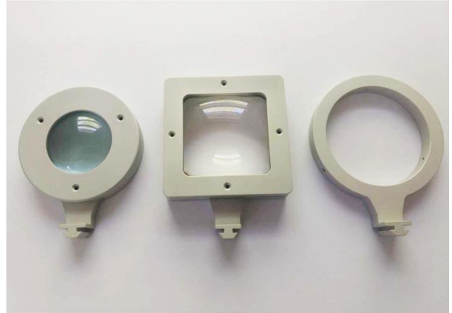
Fig. 11. Condensing lens system – lens holders 3D modelled, milled in aluminium and anodised.
