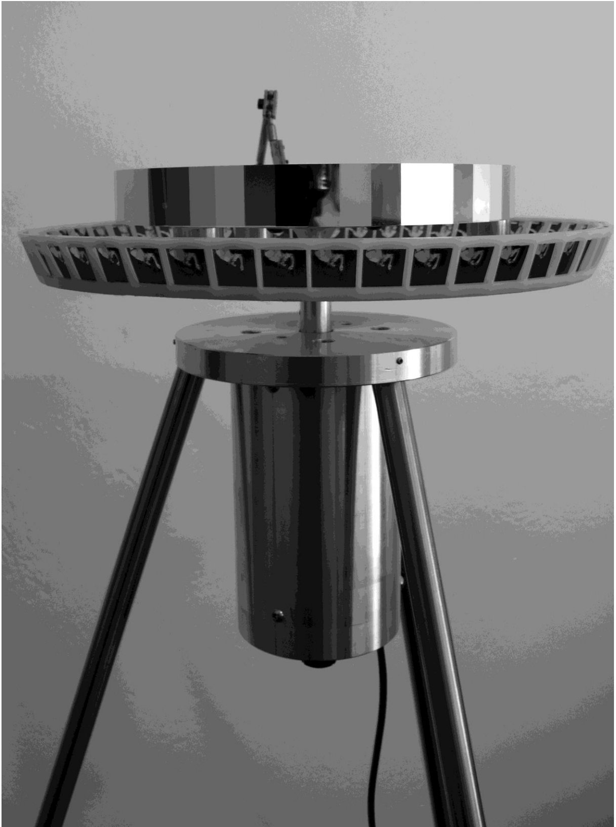
Fig. 45. Polished aluminium polygon and nylon image carousel on aluminium tripod stand.
