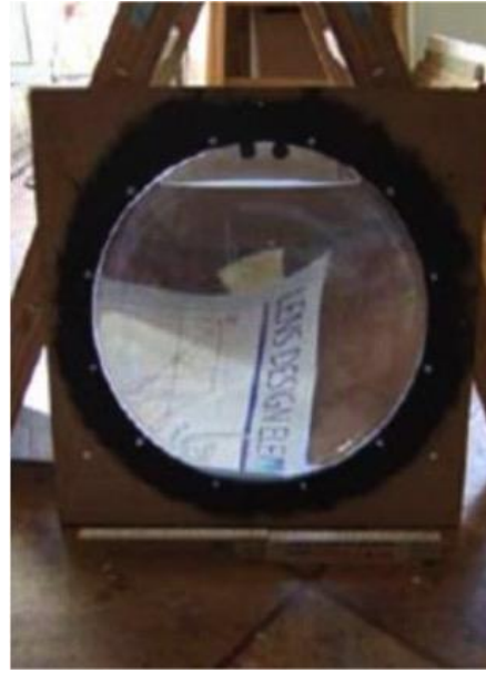
Fig. 15. Carsten Wirth. Assembled hollow lenses with water. Max Plank Institute for the History of Science, Berlin, 2007.
