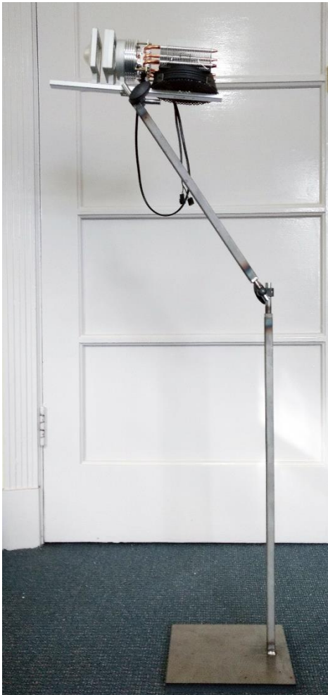
Fig. 20. LED and lens armature.
