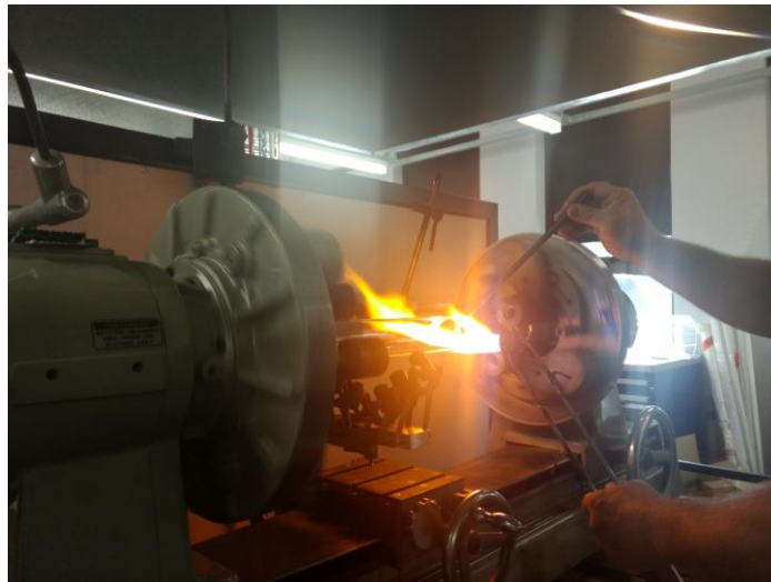
Fig. 23. Hollow lenses being blown on a glass lathe.
