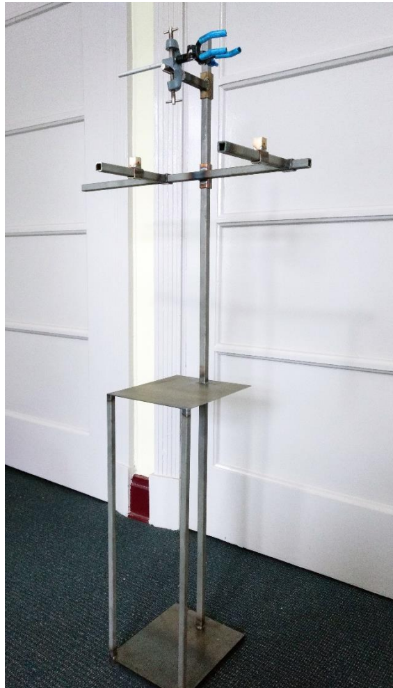
Fig. 21. Stand for the water lenses.
