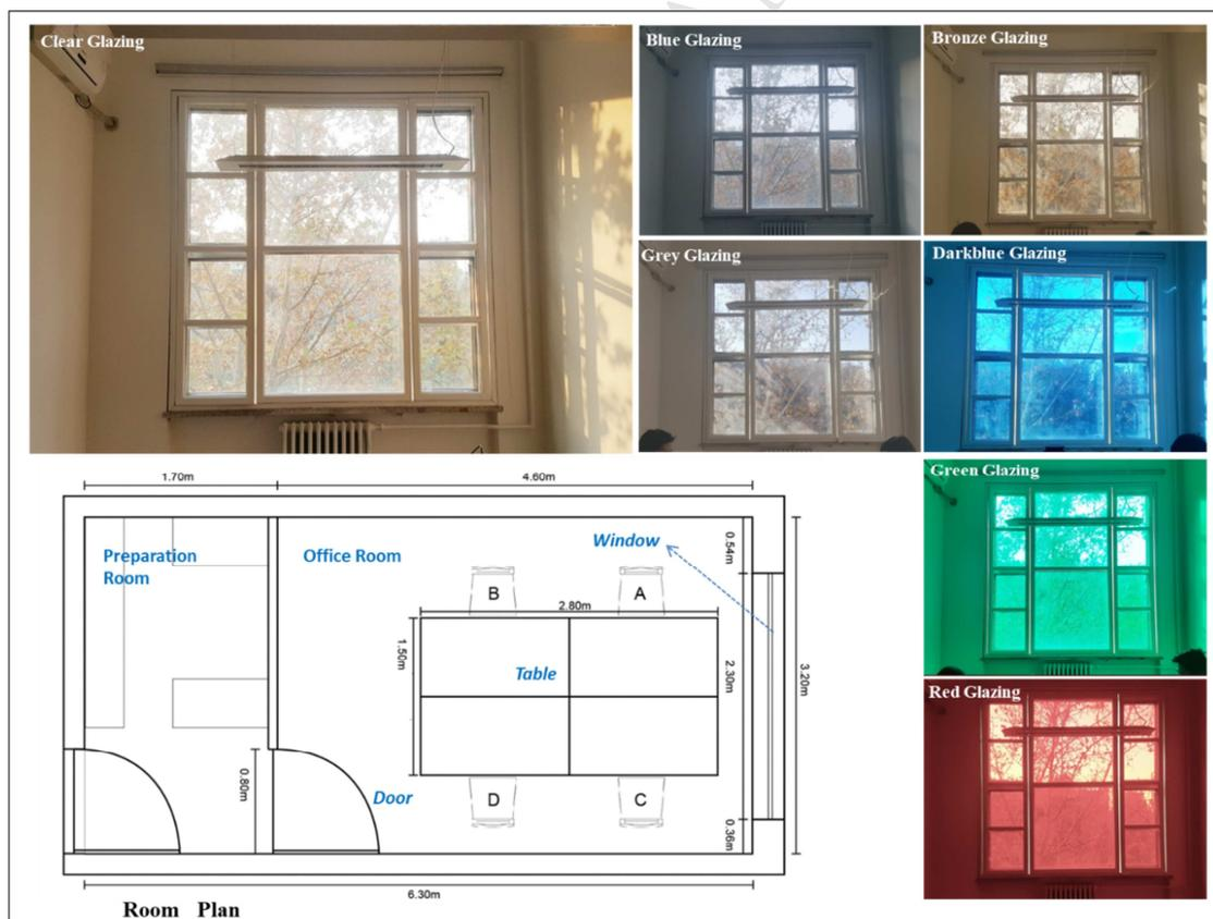
Figure 1. Plan and dimensions of the room studied, and interior views of seven coloured glazing windows.
