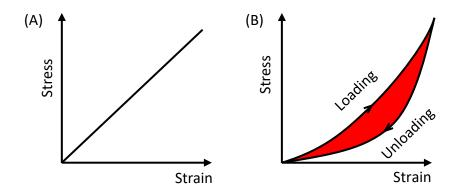
Figure 2-20 Stress-strain curves for a purely elastic material with no hysteresis (A) and a viscoelastic material with hysteresis (B). The red area shows the amount of energy lost in a loading and unloading cycle, which is an indication of the magnitude of hysteresis.
