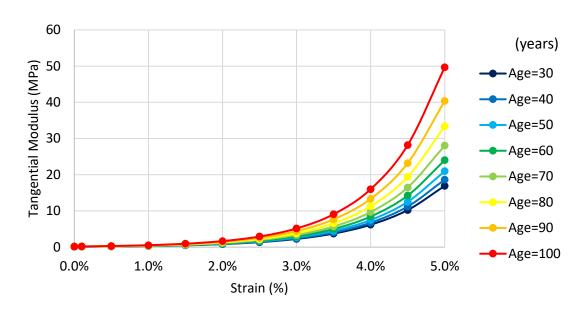
Figure 2-4Tangential modulus-strain relationships of corneal material with different Ages [1]
