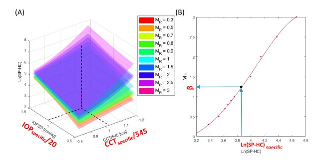
Figure 3-21 The process of corneal material estimation. (A) When specific values of CCT (CCT<sub>specific</sub>) and IOP (IOP<sub>specific</sub>) are applied in the SP-HC surface plot, there are several estimates for SP-HC for different  $M_R$ . (B) When these estimates are plotted,  $\beta$  can be estimated using the corresponding SP-HC (Ln(SP-HC)<sub>specific</sub>).
