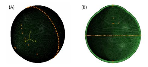
Figure 3-12 View of a FEM showing (A) full eye model and (B) cross-sectional view.
