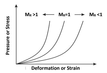
Figure 3-19 Comparison of the effect of M<sub>R</sub> value on the loading-deformation and stressstrain behaviour
