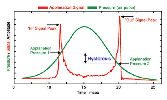
Figure 2-18 Typical light signal (red) and pressure signal (green) versus time [195, 197]
