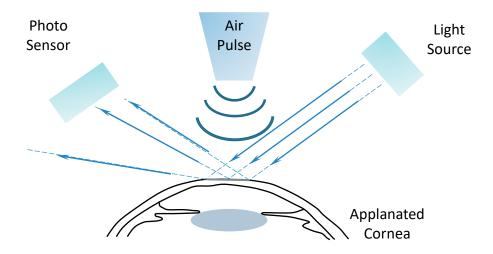
Figure 2-15 Principles of non-contact tonometry (NCT) [192]
