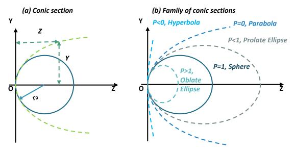
Figure 3-10 General Equation for a general conic section (a) is given by  $Y^2=2r_0Z-pZ^2$  and the family of conic sections with different asphericities is shown in (b) [235]
