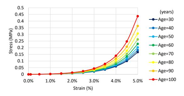
Figure 2-3 Stress-strain relationships of corneal material with different Ages [1]
