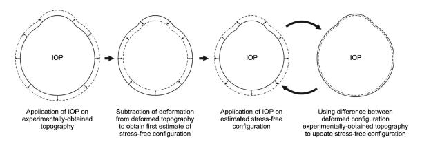
Figure 3-14 Schematic description of the approach used to obtain the stress-free configuration of the eye [233]
