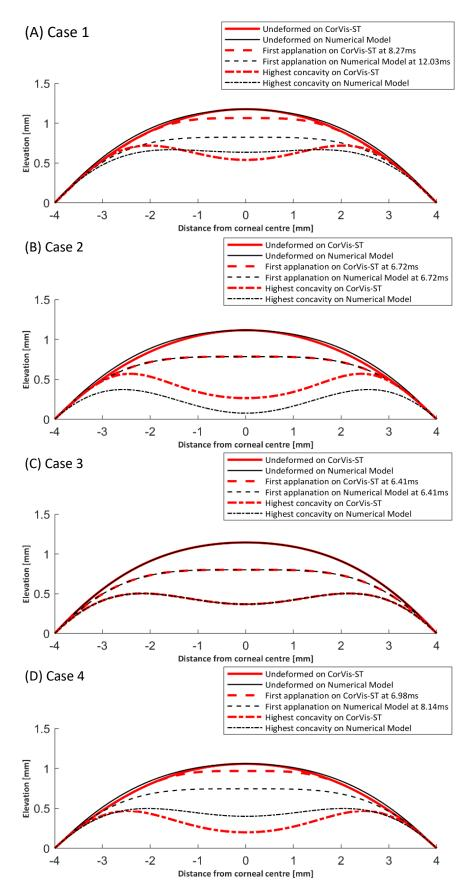
Figure 4-1 Comparison of numerical predictions with clinical measurements of corneal deformation at the start of the analysis, first applanation and highest concavity
