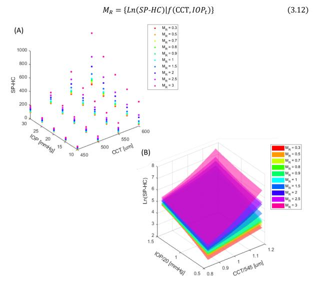
Figure 3-20 (A) 3D point cloud plot and (B) surface plot of corneal stiffness parameter against IOP and CCT for different M<sub>R</sub> values
