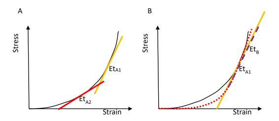
Figure 2-6 Tangent modulus of material with non-linear behaviour: (A) Tangent modulus varies with stress; (B) Tangent modulus in constant one zone of linear behaviour at different non-linear material behaviour.
