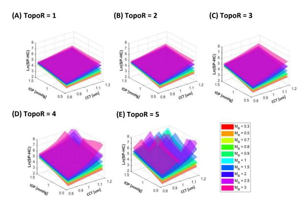
Figure 3-22 3D surface plots of stiffness parameter against IOP/20 and CCT/545 for different TopoR. Every surface corresponds to a specific value of  $M_R$ .
