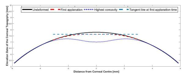
Figure 3-16 Corneal anterior profiles during air-puff loading
