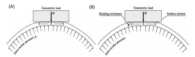
Figure 2-14 Comparison between principles of (A) Imbert–Fick law and (B) Goldmann
