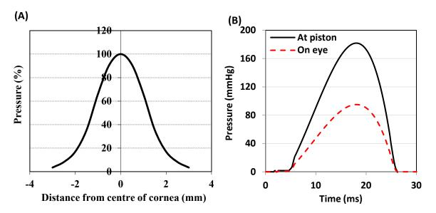
Figure 3-13 Spatial distribution (A) and time variation (B) of air-puff pressure on the cornea [46, 242, 243]. In (B), thick black line represents pressure measured in device piston and the red line represents pressure acting on the cornea.
