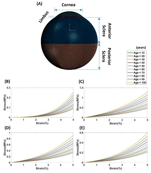
Figure 3-11 Model segments with different material properties in FEM (A). Stress-strain material behaviour of the cornea (B), limbus (C), anterior sclera (D), and posterior sclera (E) with age-related variation is shown [1, 70].
