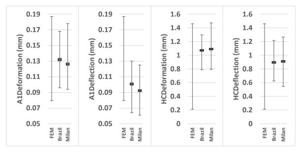
Figure 4-2 Ranges of dynamic response parameters - deformation and deflection at the first applanation and highest concavity in numerical predictions compared to the boxplot indicating the mean, range and confidence interval ranges at p=95% for the CorVis-ST output in two clinical datasets (Brazil and Milan) for healthy eyes
