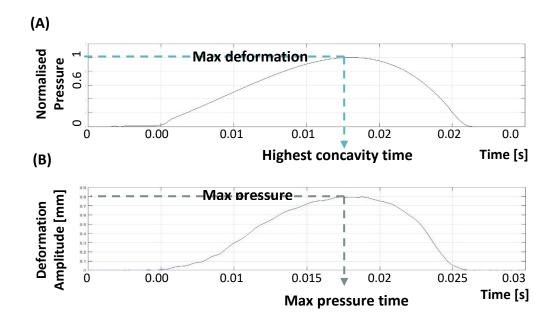
Figure 3-15 Progress of normalised air pressure (A) and nodal deformations at the corneal apex (B) with time. When air-puff pressure increases to a maximum, corneal apex deformation reaches its max value.
