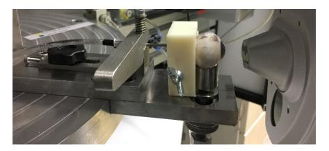
Figure 3-24 Test rig showing eye sitting on a rigid support and supported from the back while being connected to a syringe pump that controls its IOP. CorVis ST is placed at a distance to enable its automatic trigger.
