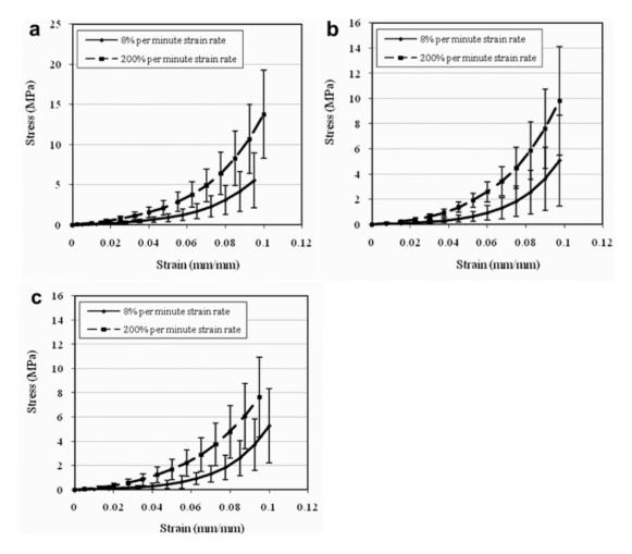
Figure 2-5 Strain rate effects on average stress-strain behaviour of scleral tissue in (a) anterior, (b) equatorial and (c) posterior region [70]
