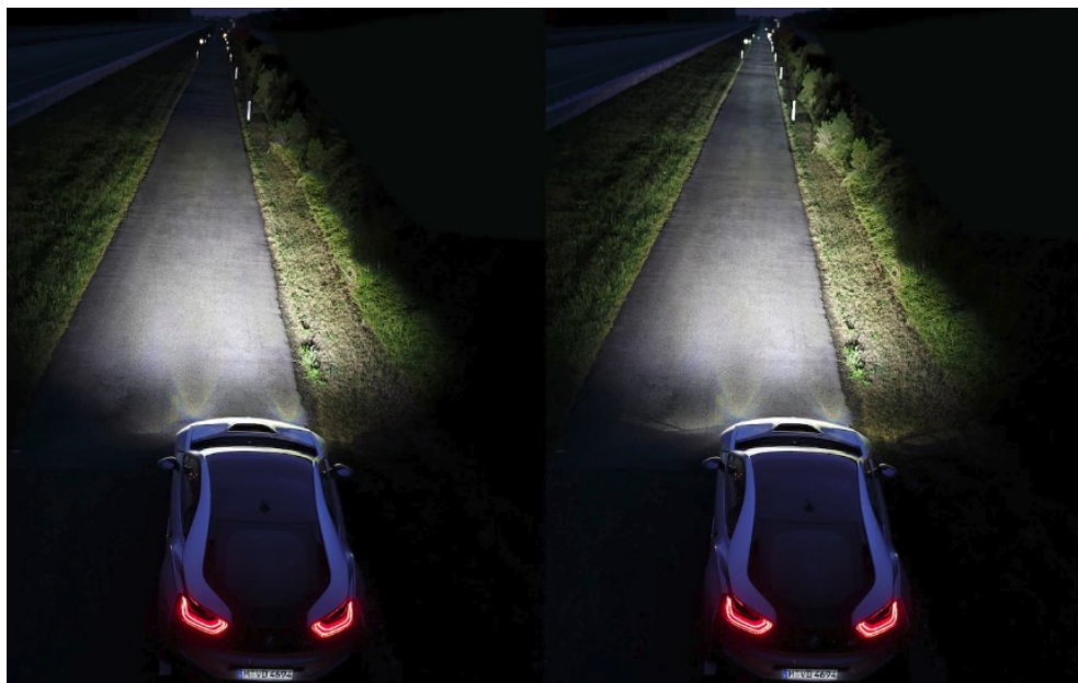
Figure 2.8: Laser headlights (right) offer increased visibility compared to LED headlights (left) [92].
