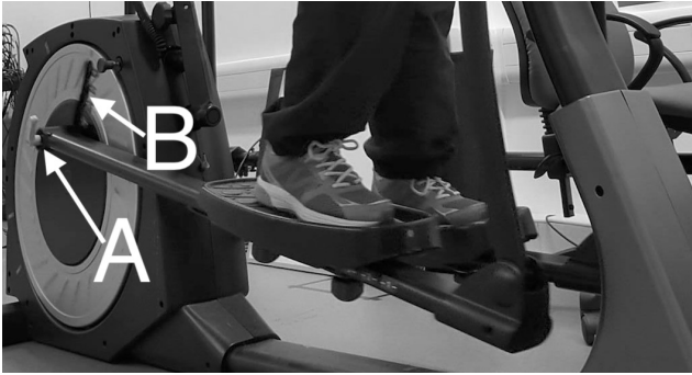
Figure 1: The height (difficulty) of FRED’s walking path is increased by moving the rear end of the stride rail (A) through the slot (B) towards the edge of the wheel. FRED has five such settings and is shown here in its default (lowest) configuration.
