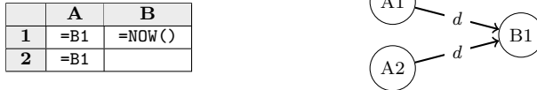
Fig. 5 Two cells depend on the same cell containing a call to NOW() . If both cell A1 and A2 are evaluated in parallel and both recursively attempt to evaluate B1, their respective threads must agree upon which value B1 has evaluated to
