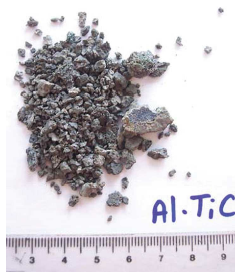
Fig. 5 – Al/TiC master alloy produced by SHS containing 40 wt.% of pure free aluminium manually crushed before the ball milling process.
