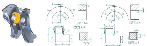
Figure 7. Description of the defects manufactured on complex specimens
