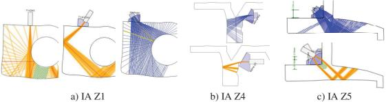
Figure 10. Results from simulations identifying non-inspectable areas (in green).
