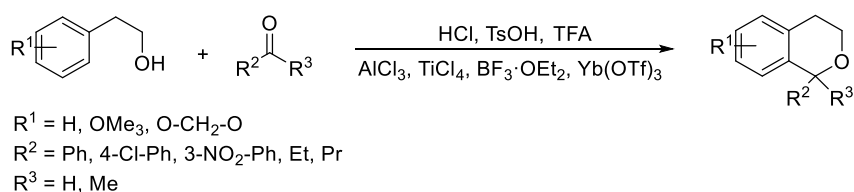
Scheme 45. Synthesis of 1-substitued isochromans via oxa-Pictet-Spengler reaction.
