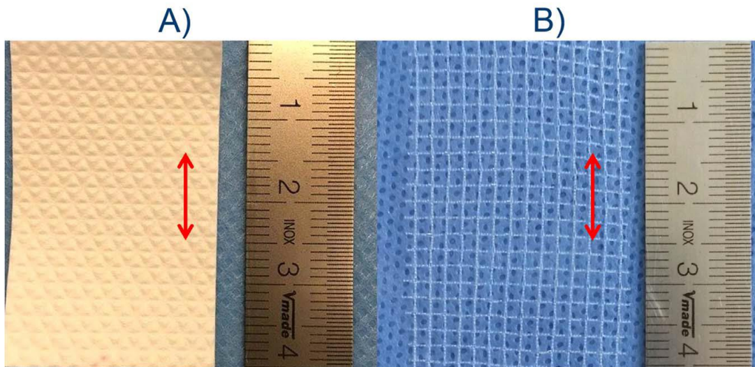
Fig. 1 Implanted materials: A: UPy-PCL electrospun and B: Restorelle®. Red arrows indicate the direction of loading for the ex vivo mechanical characterization of the implants under dry and wet conditions. (For interpretation of the references to colour in this figure legend, the reader is referred to the web version of this article.)
