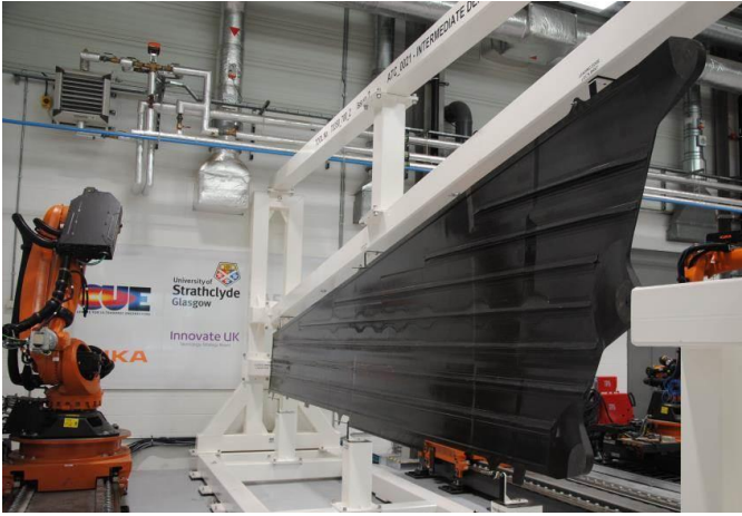
Fig. 1. Multi-robot flexible inspection at the University of Strathclyde
