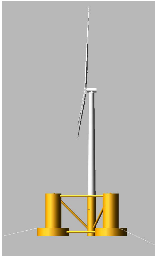
73 74 Fig. 1. DeepCwind floating wind turbine system design (Coulling et al., 2013).
