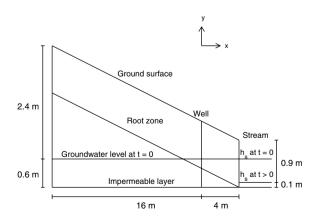
**Figure 2** Schematic vertical cross-section of the aquifer employed in the numerical model. The left-side of the aquifer represents no-flow conditions, and the fully incised stream ( $h_s$  is stream stage) is on the right-side of the aquifer.
