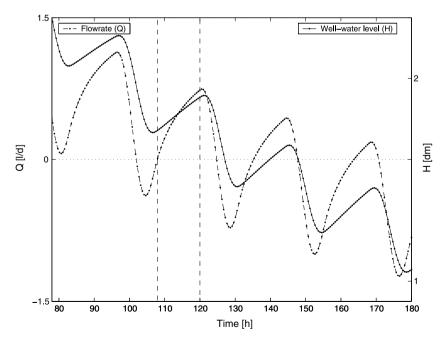
**Figure 3** Modeled aquifer outflow, Q, and well-water level, H, time series in the second part of the 8-day drawdown with a constant stream-water level of 0.1 m for t > 0. The first vertical line denotes the end of the previous ET cycle at hour 108 and the second one denotes the start of the following one at hour 120, for easier interpretation.
