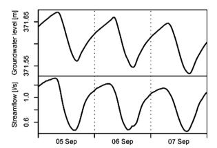
**Figure 1** Observed diurnal fluctuations in the riparian zone groundwater-level and streamflow values at the Hidegvíz—völgy experimental catchment of north-western Hungary (from Gribovszki et al., 2008).
