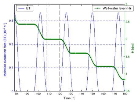
**Figure 4** Spatially uniform moisture extraction rate that corresponds to a daily ET rate of 2 mmd<sup>-1</sup> from a flat, 1 m thick aquifer with a root zone of 1 m in depth and initial water level of 0.6 m. The dots denote the elevation of the groundwater-surface at the "well" 4 m from the right edge. The aquifer now has no-flow boundaries at either side.
