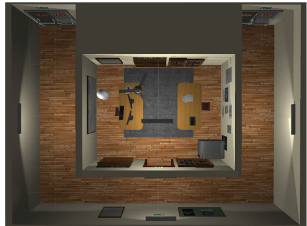
Fig. 5 Bird's eye view of building layout: room with corridors leading to two possible emergency exits
