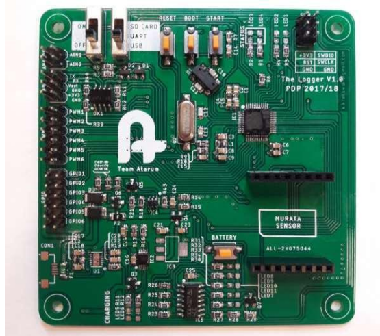
Figure 51 Custom printed circuit board for the data logger (Self Elaborated)
