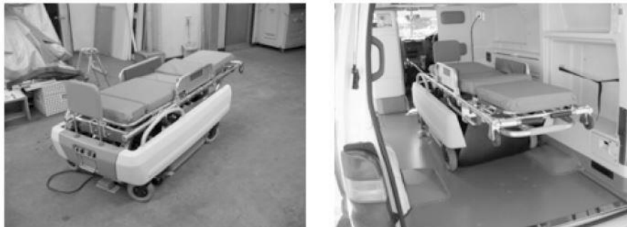
Figure 21 2-degree-of-freedom (2DOF) prototype of actively controlled bed [47]
