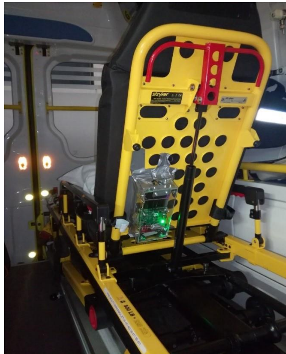
Figure 50 Data logger mounted to the stretcher (Self Elaborated)
