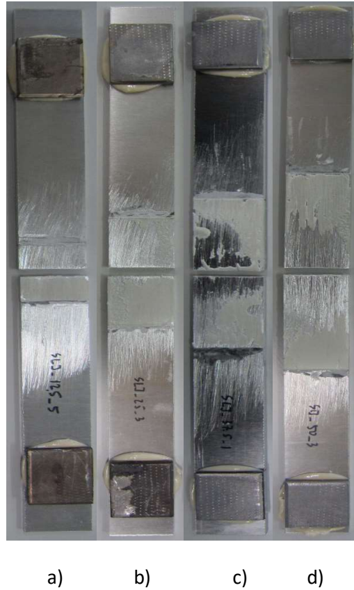
Figure 56 - Failure modes of the specimens bonded with the adhesive Sikaforce®7752, and L_0=12.5 (a), 25 (b), 37.5 (c) and 50 mm (d)
