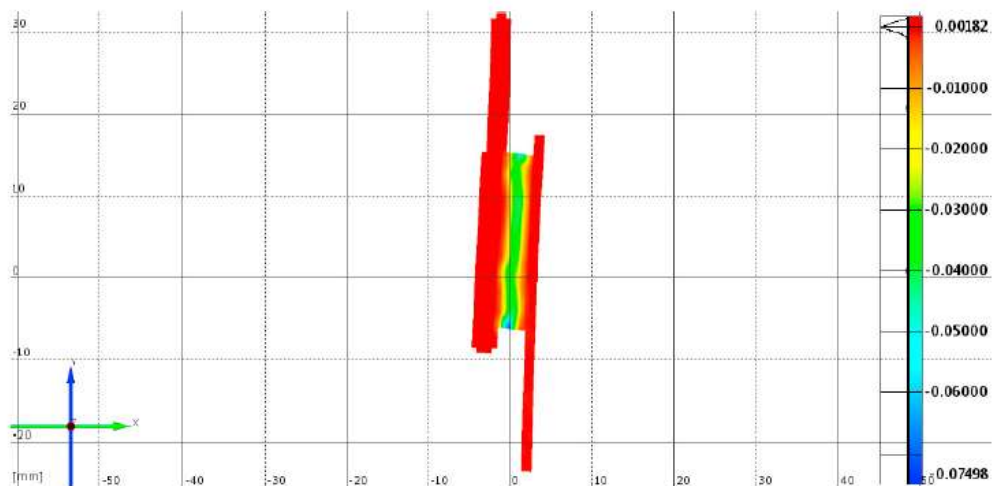
Figure 26 - Shearing strains in the adhesive for an aluminum-carbon joint [57].
