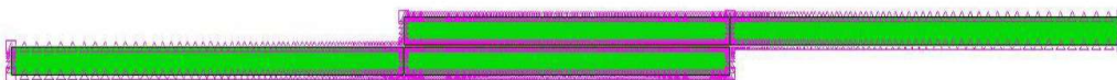
Figure 68 - Bias effect of the mesh in the unbound region of the adhesives for SLJ
