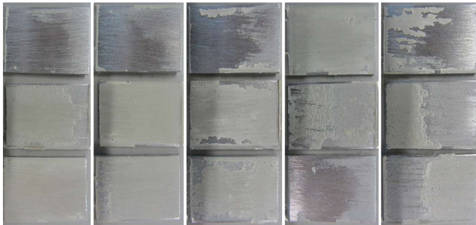
Figure 62 - Failure modes of DLJ specimens bonded with the adhesive Sikaforce®7752 L_0=50 mm.
