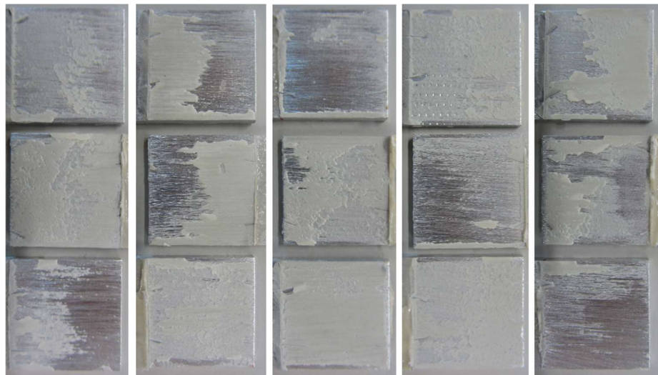
Figure 60 - Failure modes of DLJ specimens bonded with the adhesive Sikaforce®7752 L_0=25 mm.
