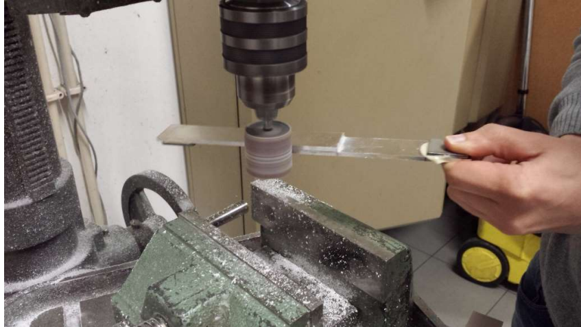
Figure 46 - Adhesive excess removal [65]
