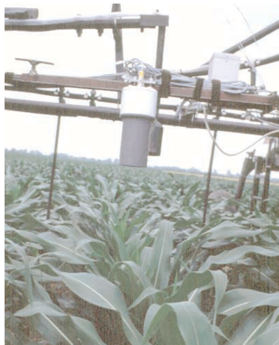
Figure 42. A spectral radiometer mounted on a variable-rate applicator can reduce overapplication while delivering nitrogen fertilizer where it is needed.
