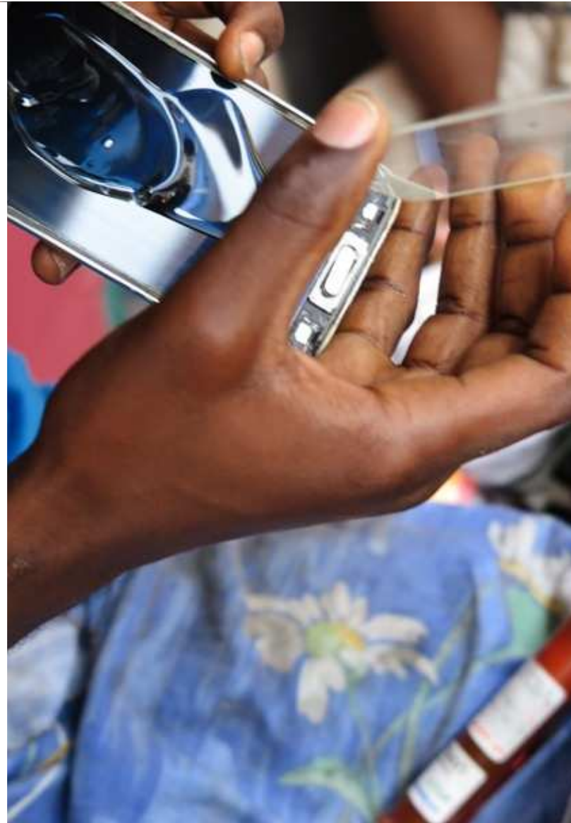
Adding the right amount of glue to fasten the new glass
