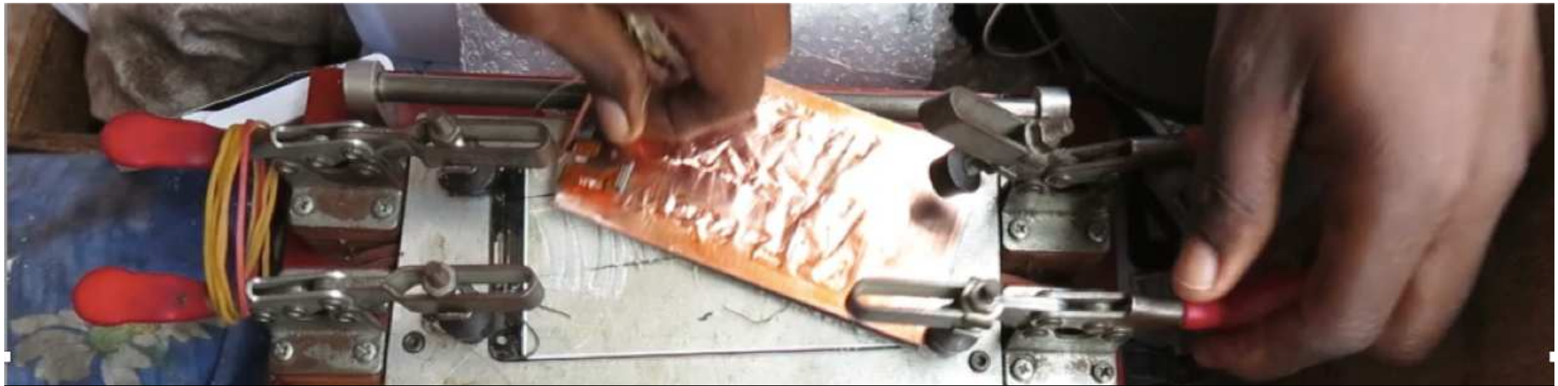
separating the broken glass from the display unit
