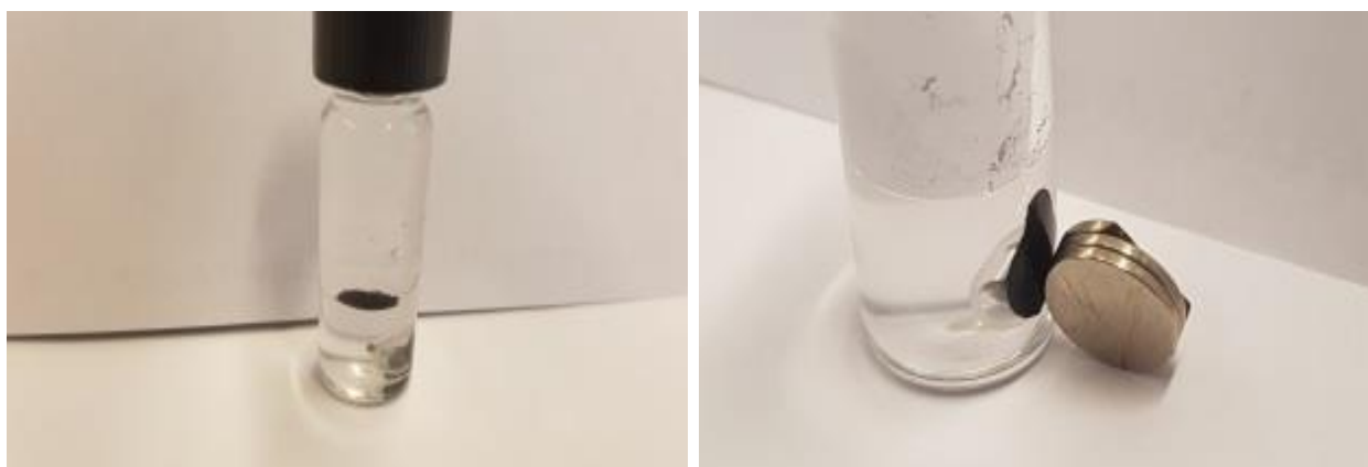
Fig. S1. Recycling of Co@Chitosan-700. Left: Vial containing the reaction mixture with catalyst. Right: The catalyst is attracted by a magnet. Photo Credit: Florian K. Scharnagl, Leibniz-Institut für Katalyse e.V. an der Universität Rostock
