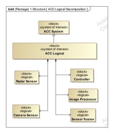
Figure 4.13.: SysML bdd for 'ACC Logical Decomposition'
