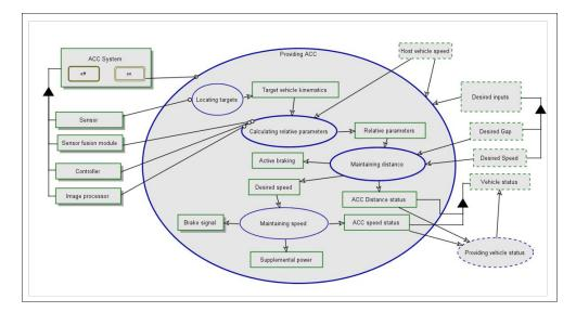
Figure 3.6.: Object-Process Diagram for SD1: 'Providing ACC' in-zoomed
