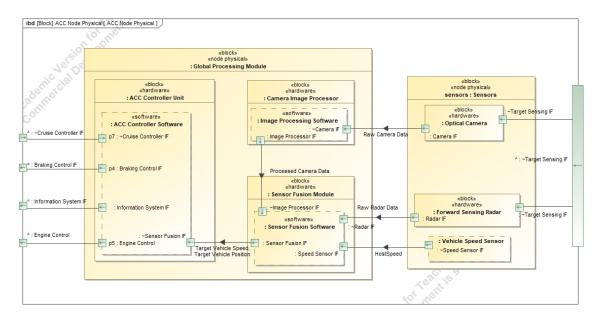
Figure 4.19.: 'ACC Node Physical Architecture' using SysML ibd
