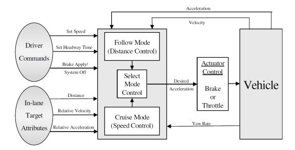
Figure 3.2.: ACC control structure [48]
