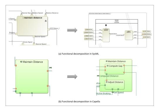
Figure 5.2.: Function decomposition in SysML and ARCADIA/Capella
