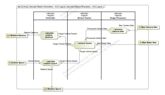
Figure 4.14.: SysML *activity diagram (act)* for 'calculate relative parameters' function
