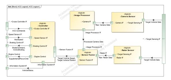
Figure 4.15.: 'ACC System Logical Architecture' using SysML ibd
