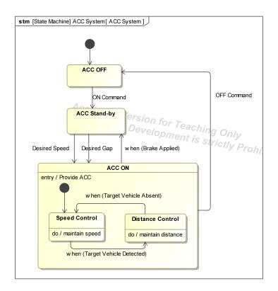
Figure 4.11.: SysML state machine diagram (stm) for 'ACC System States'
