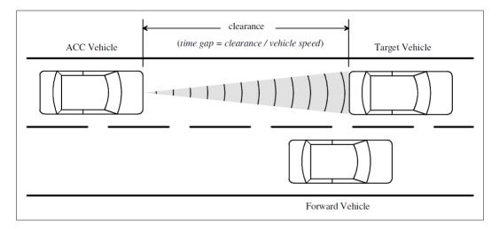
Figure 3.1.: ACC-equipped vehicle external relationships [46]
