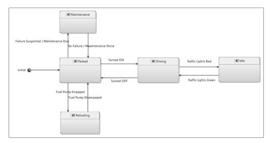
Figure 4.25.: 'Vehicle Operational States' using Mode State Machine [MSM] diagram
