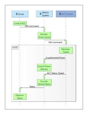
Figure 4.32.: 'Turn ACC ON' exchange scenario using the *Exchange Scenario* [ES] diagram
