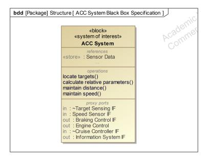
Figure 4.10.: ACC System Black Box Specification
