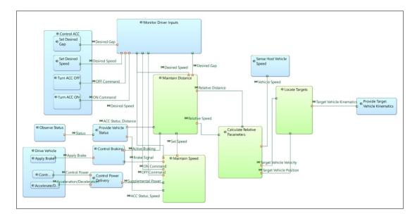
Figure 4.29.: 'Provide ACC' functions modeled using System Data Flow Blank  $[SDFB]\ diagram$
