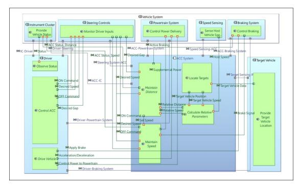
Figure 4.31.: 'ACC System Architecture' using the System Architecture Blank [SAB] diagram
