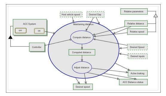
Figure 3.10.: Object-Process Diagram for SD1.2: 'Maintaining distance' in-zoomed
