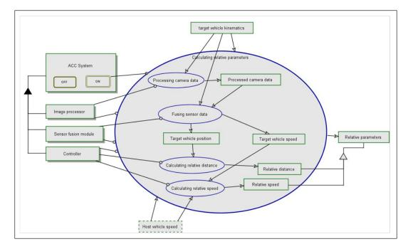
Figure 3.8.: Object-Process Diagram for SD1.1: 'Calculating relative parameters' in-zoomed
