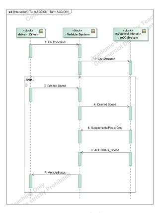
Figure 4.6.: SysML sequence diagram (sd) for 'Turn ACC ON' scenario
