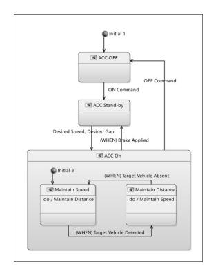
Figure 4.33.: 'ACC System States' using Mode State Machine [MSM] diagram
