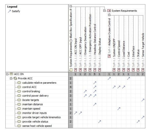
Figure 5.3.: Satisfy Requirement Matrix in Cameo Enterprise Architecture
