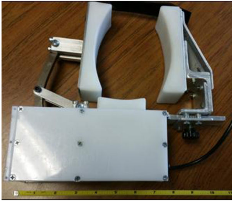
Figure 1. Knee loading device with a voice coil linear actuator.
