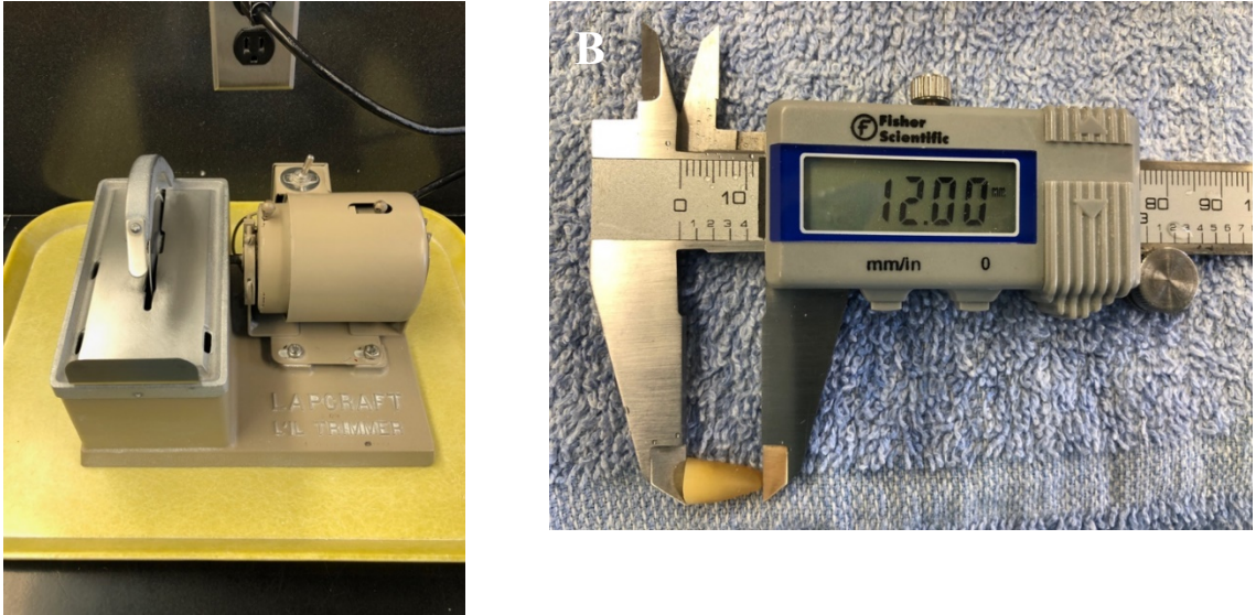
FIGURE 3. Diamond saw (A) used to standardize roots to 12 mm (B).
